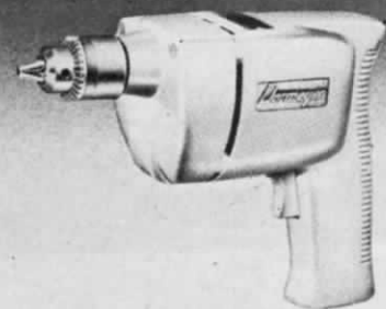
No. 210 — ¼" DRILL WITH FAMOUS GEARED CHUCK. Die cast aluminum alloy housing. Self lubricating bearings. Multiple ball thrust bearing. Capacity in steel, ¼"; ½" in hard wood. No load speed, 1800 RPM. 115V. AC-DC. Automatic shut-off, built-in lock. 8¾" long. LIST $24.95.
